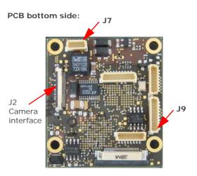
J2: FCB-EV, -EH, -SE 30pin LVDS connector J1,J3,J8: not assembled J9: RS232 UART connector J7: External power connector (arrow marks pin 1): Pins 1, 2: Input voltage 5V to 7V DC Pins 4, 5: GND Pin 3: System reset, pull to GND for reset J4, J5, J10: do not connect
